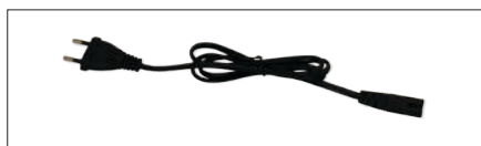
PSD12 Kabel 230VAC 2x 0.5 mm², 1,2 m, CEE 7/16, IEC C7
